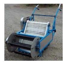
mechanical harvester to which they have made numerous adjustments to reduce damage to the berries. Regardless of which method is used for harvesting, the operator can 'make or break' the berry quality depending on how they handle the machine
