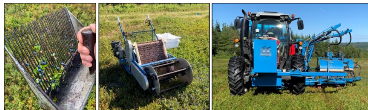
Figure 1: Harvesting of wild blueberries with the help of (left) a hand-held metal rake, (center) walk-behind harvester, and (right) a DBE mechanical harvester.
