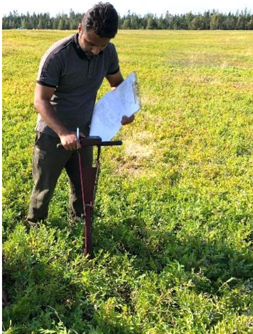
Figure 6: Determining of (a) soil moisture levels with a Time Domain Reflectometry probe TDR-300 and (b) photosynthetically active radiations (PAR) above and below the plant canopy using a PAR external sensor.
