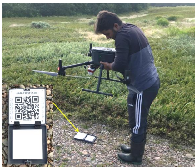
Figure 14: A drone MicaSense Altum sensor connected with a drone (a) was calibrated (b) prior to and after each flight.
