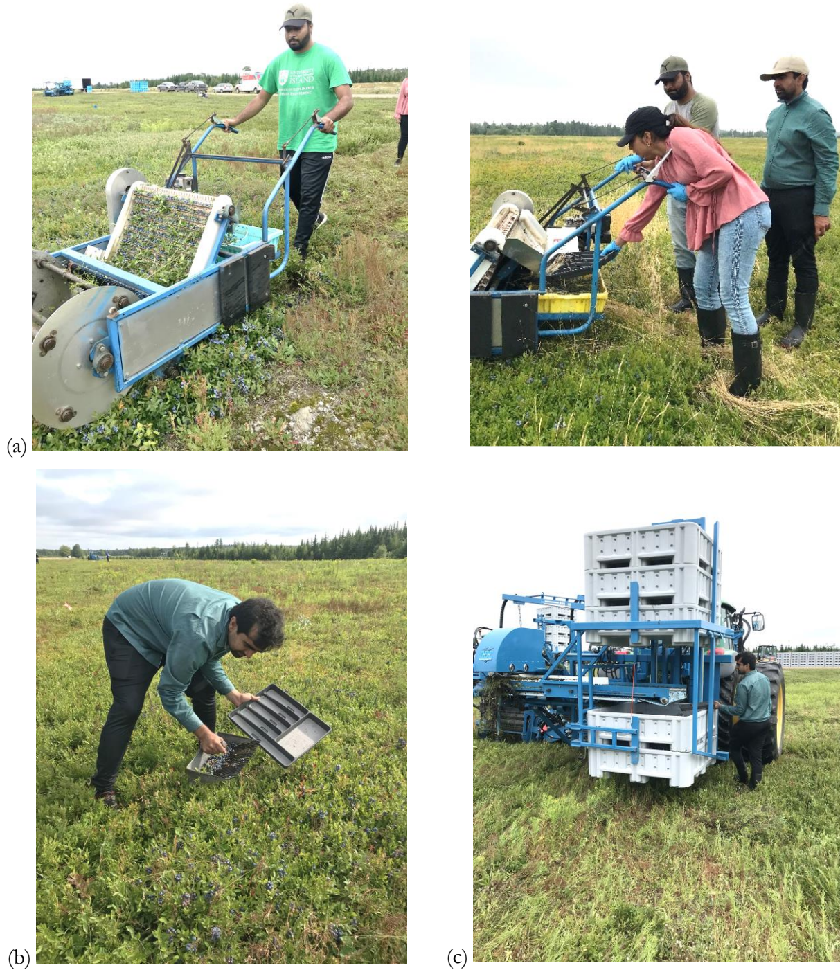
Figure 7: Collection of berry harvest samples with (a) walk-behind manually operated harvester (b) hand raking, and (c) Doug Bragg Enterprises mechanical harvester.
