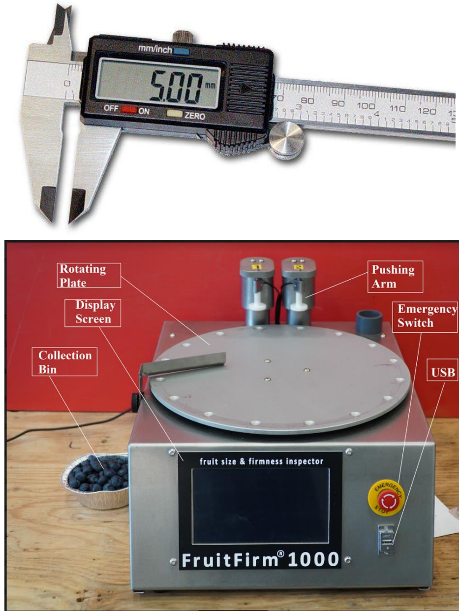
Figure 11: A vernier caliper (top) and FruitFirm 1000 instrument (bottom) to measure fruit diameter and firmness, respectively.
