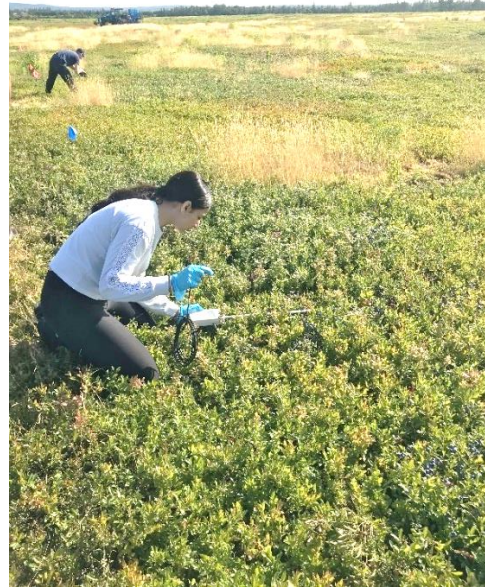
Figure 6: Determining of (a) soil moisture levels with a Time Domain Reflectometry probe TDR-300 and (b) photosynthetically active radiations (PAR) above and below the plant canopy using a PAR external sensor.
