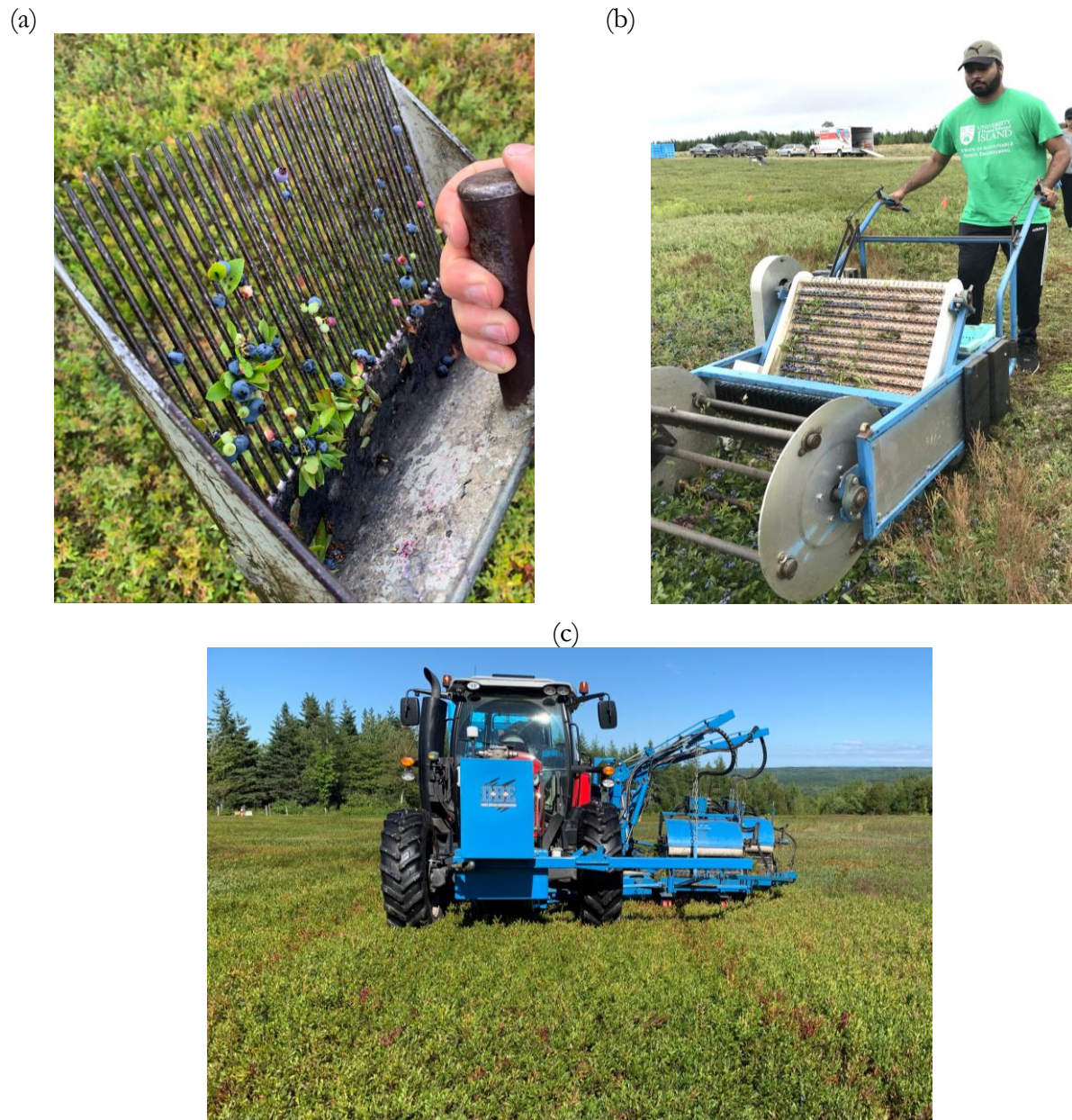
Figure 2: The tools and methods used to harvest wild blueberries included (a) hand-held metal rake, (b) manually controlled but a motor-operated walk-behind harvester and (c) a Doug Bragg Enterprises mechanical harvester mounted on a farm tractor.
