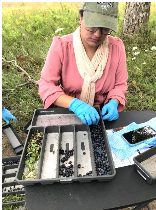
Figure 8: Temporary arrangements for segregating raw harvest samples into i) good berries, ii) bruised berries, iii) cut-split berries, and iv) debris.
