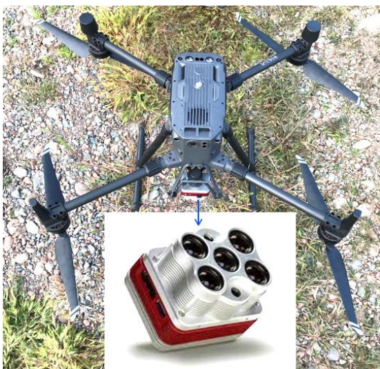
Figure 14: A drone MicaSense Altum sensor connected with a drone (a) was calibrated (b) prior to and after each flight.
